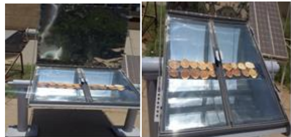
Fig. 4 A photographic view of the baked bread inside the PTB. The eight thermocouples are distributed inside the PTB to measure the temperature of the air enclosure and the receiving absorber plate as shown in Fig. 5.
